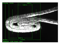
During the inspection process, SeamMate<sup>®</sup> software automatically calculates seam tightness by analyzing the geometry of captured seam images.
